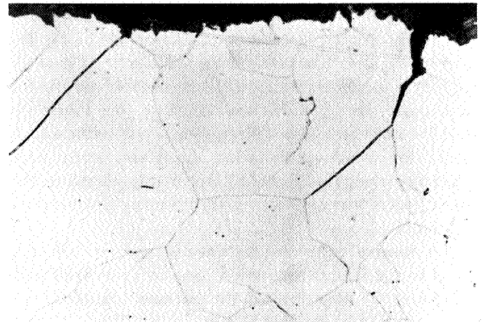
Figure 7. Surface cross section of bellows; 1-min. picral-HCl etch (Mag. 1000X).
